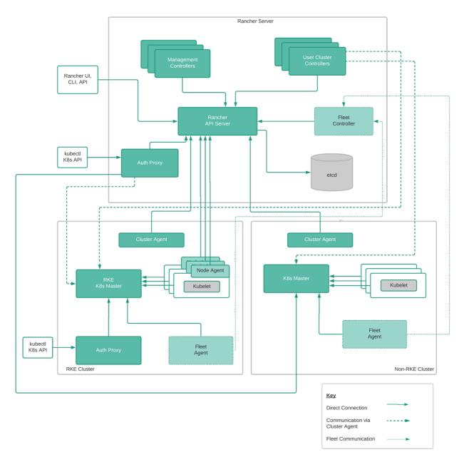
Figure 2: SUSE Rancher 2.6 High-Level Architecture
